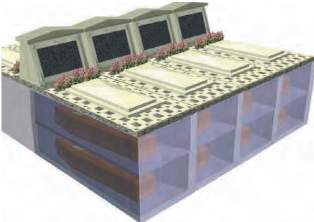
Double depth below ground burial chambers with memorial systems
